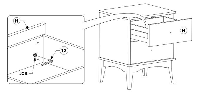
After the Drawer Faces (H) are aligned, secure with wood screws.
